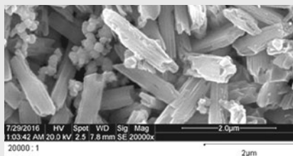
Conventional LS_2 Press ingot HT A2 Etched surface (Lithium Disilicate crystal ~ 1.8 \mu\text{m} )
